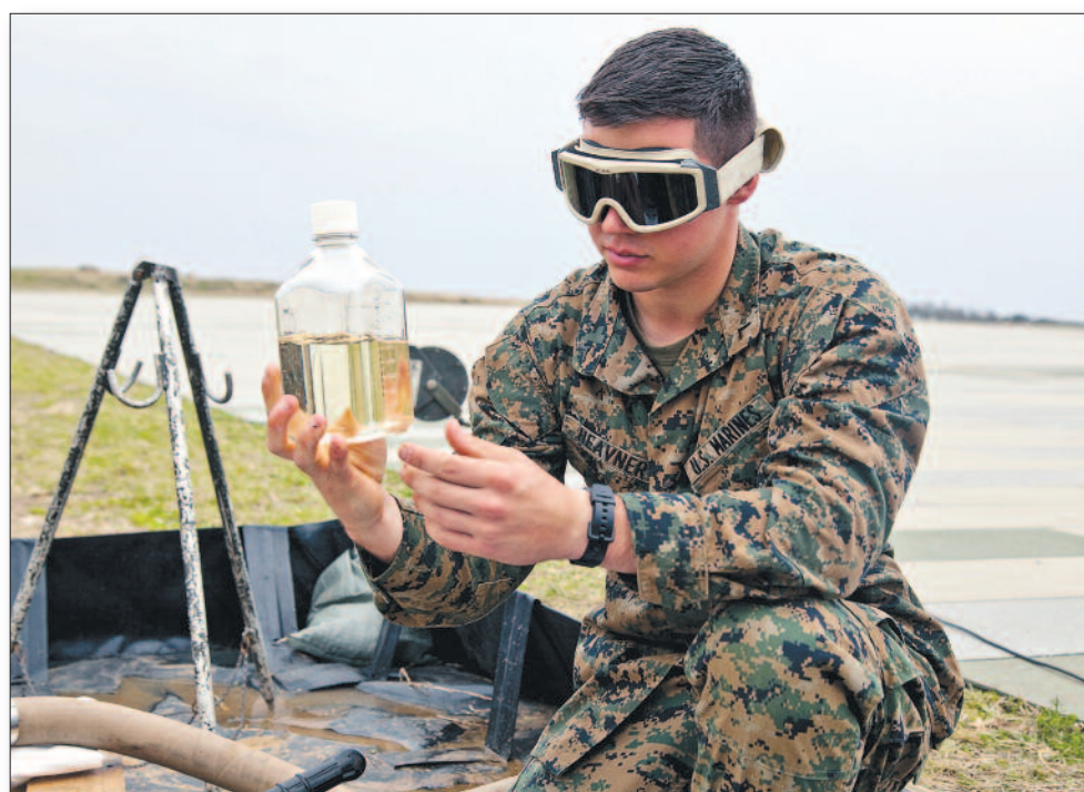
Pfc. Colby J. Heavner, bulk fuel specialist, Marine Wing Support Squadron 172, Marine Aircraft Group 36, 1st Marine Aircraft Wing, III Marine Expeditionary Force, takes a fuel sample during bulk refueling training Jan. 16 at Ie Shima training facility on Okinawa, Japan. The samples are used to test the fuel potency and check for contaminants to ensure the aircraft receive high-quality fuel.
